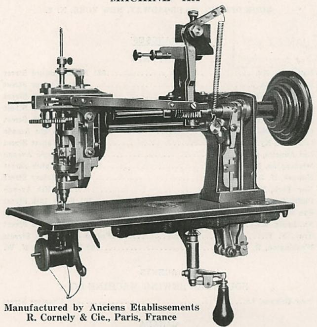
This machine has an Automatic Attachment, by means of which it is possible to produce certain designs of embroidery automatically by means of cams and without skilled operator.
