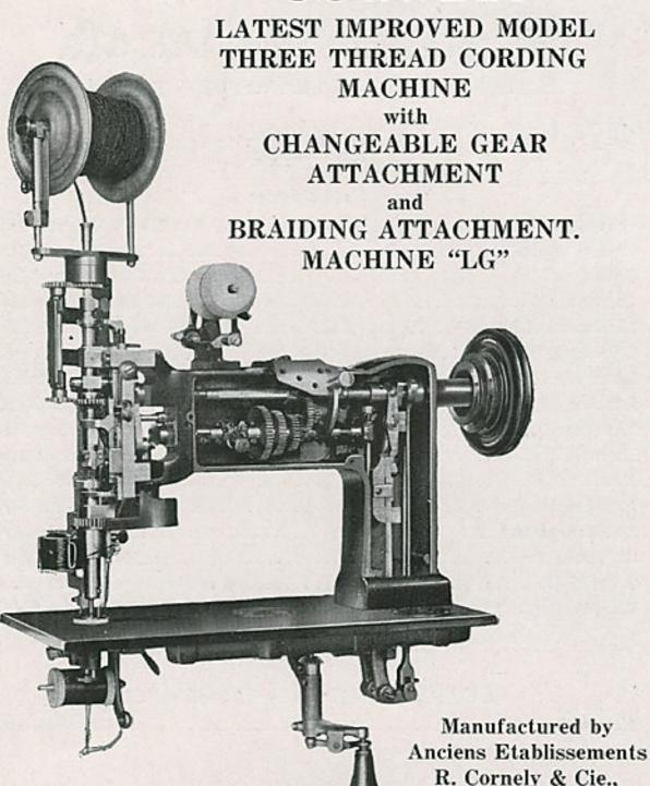
This machine is the latest progression and improvement of the Cornely Machine L, having a built-in Changeable Gear Attachment by means of which the revolutions of the Cording Spool Carrier can be retarded in its action instantly, to make one revolution to each One, Two, Three, Four, Five or Six stitches of the needle.
