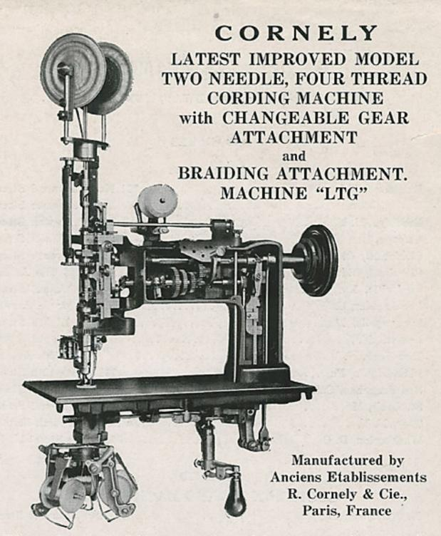
This machine is the latest progression and improvement of the Cornely Machine LT, having a built-in Changeable Gear Attachment by means of which the revolutions of the Cording Spool Carrier can be retarded in its action instantly to make one revolution to each One, Two, Three, Four, Five or Six stitches of the needle.
