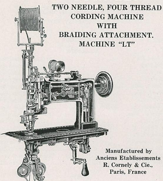
This machine works with two needles, which produce two rows of parallel chain stitches. A third thread is wound around the two chain stitches and thus produces embroidery or edging stitches, the thickness of which can be varied according to the thickness of the filling which passes through the central tube.
