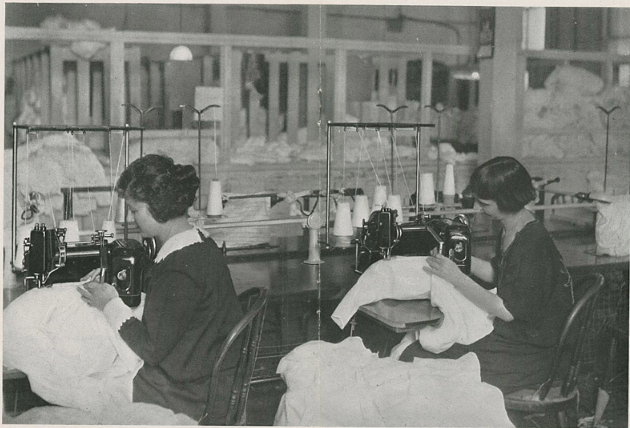
"Feldlock" Machines feed OFF the cylinder instead of ONTO the cylinder, thus increasing production
