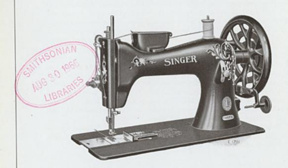
This machine is very strongly built and is specially designed for stitching heavy textiles such are used in the manufacture of small Canvas Driving Belts, Cocoa-matting, Rugs, Sacks, Travelling Bags, Horse Clothing, Awnings, Sails, Tarpaulins, Wagon Covers, Tents, Trunk Covers, etc.
