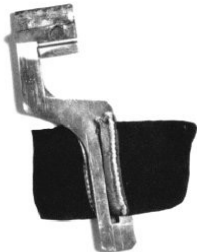
Figure 61.—SPOUL's patent braid guide, 1871. (Smithsonian photo P-63102.)
