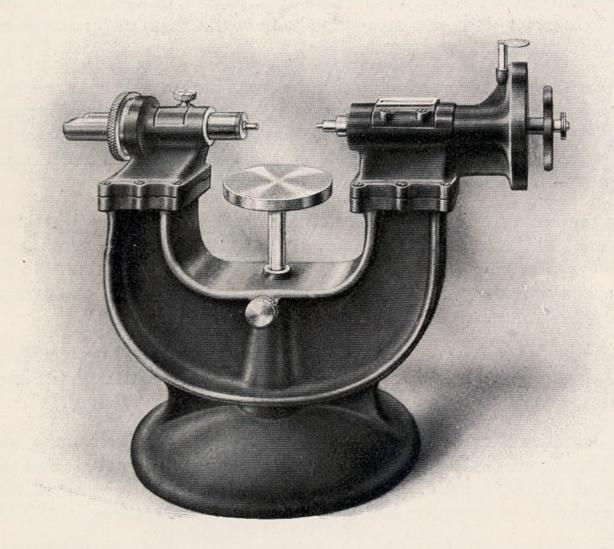
The principle of this instrument is the same as that of the ordinary Screw Micrometer, but is distinguished by its extreme accuracy and the care taken with its construction. The ample proportion of the main casting allows of its supporting heavy pieces without harmful deformation. It is provided with a table which can be adjusted vertically, so that the object to be measured may be placed conveniently between the measuring faces of the machine.
