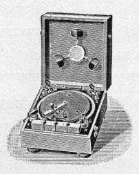
31431 Small resistance bridge with slide wire 6944
