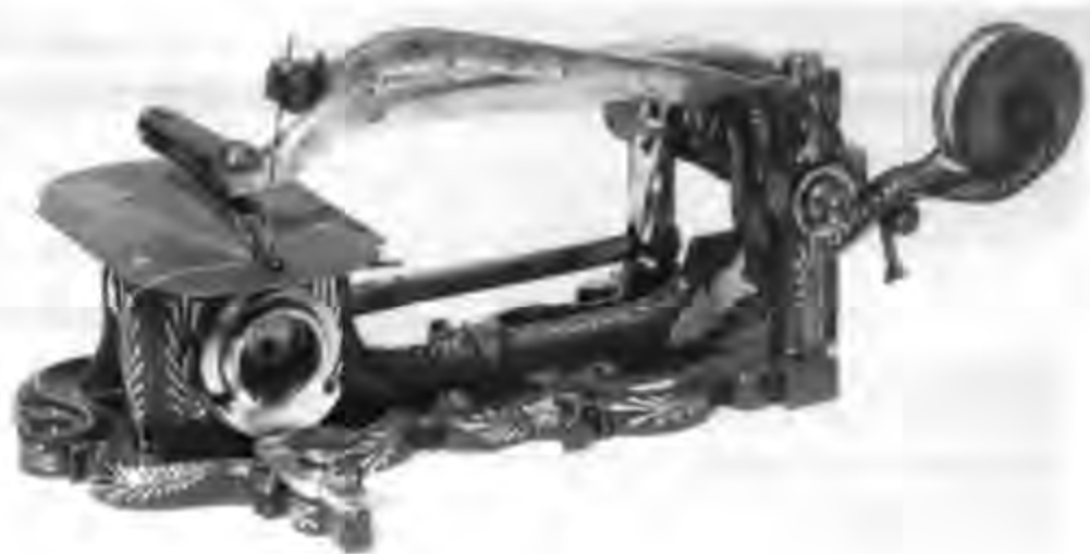
Figure 27.—WILSON'S four-motion-feed patent model, 1854, is not known to be in existence; this is a commercial machine of the period. The plate is stamped "A. B. Wilson, Patented Aug. 12, 1851, Watertown, Conn., No. 1. . . ." (Smithsonian photo 45504.)
