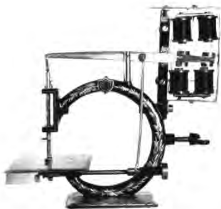
Figure 66.—JONES "ELECTRO MOTOR" PATENT MODEL of 1871 on a Bartlett sewing machine. (Smithsonian photo P-63104.)
