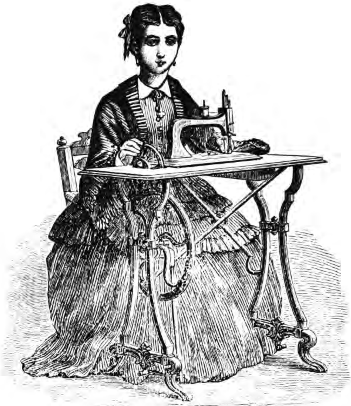
Figure 92.—GROVER AND BAKER SEWING MACHINE. The Grover and Baker machine was one of the more popular machines from the 1850s until the early 1870s. The company produced iron-frame machines, fine cabinet models, and portables (figs. 35 and 36). Their machines may be dated by serial number approximately as follows:
