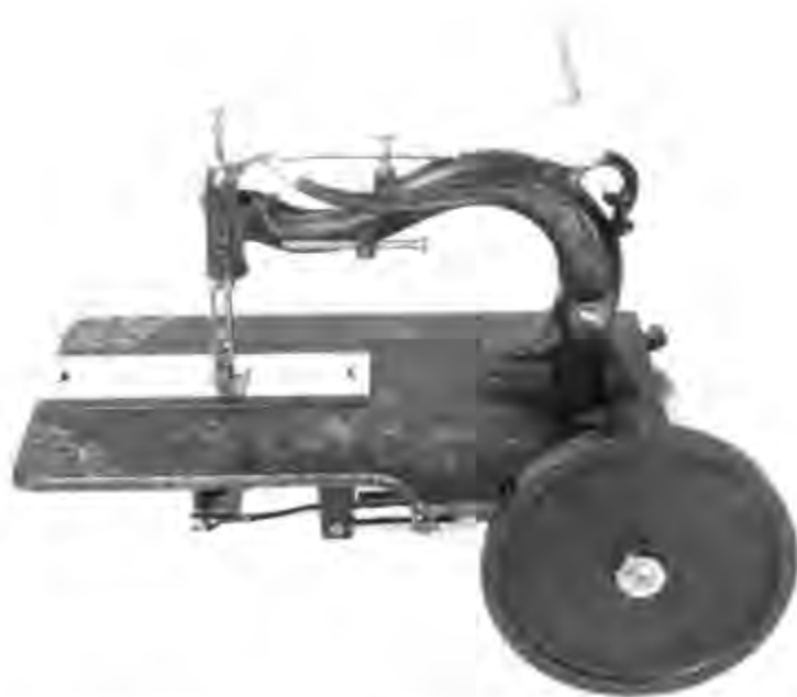
Figure 91.—GREENMAN AND TRUE SEWING MACHINE. This lockstitch machine based on S. H. Roper's patent of 1857 was manufactured at Norwich, Connecticut, from 1859 to 1861 by Cyrus B. True, the inventor, and Jared F. Greenman, True's financial partner. Licensed by the "Combination" and carrying the Howe patent date, the machine had obvious merit: it was strong, well made—a good family machine. Exhibited at the Ninth Exhibition of the Massachusetts Charitable Mechanics Association in September 1860, it received a bronze medal. (At this time the company was listed as Morse and True—the inventor had obviously taken on a second financial backer.) Unfortunately, the best market for the machine lay in the South, and the outbreak of the Civil War made collections impossible. This greatly retarded business and finally drove the firm into bankruptcy. In all, it is doubtful that more than one thousand machines were produced in the three years of manufacture.
