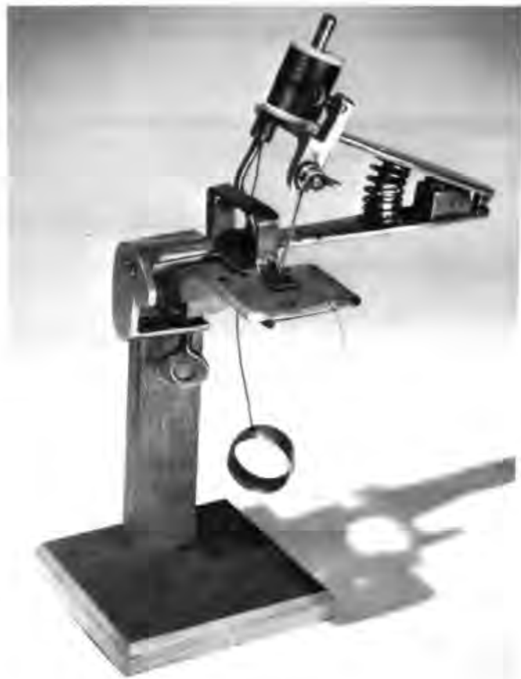
Figure 75.—BECKWITH SEWING MACHINE, 1871. Among the inventors whose patent claims were "to produce a cheap and effective sewing machine" was William G. Beckwith. His machine was first manufactured by Barlow & Son, and it realized considerable success in the few years of its production. The earliest model was operated like a pair of scissors or with a cord and ring as illustrated. Beckwith later added a hand crank. The machine was purchased in Crewe, Cheshire, England; it is stamped "Pat. April 18, 71 by Wm. G. Beckwith, Foreign Pats. Secured, Barlow & Son Manuf. N.Y., [serial number] 706." By 1874 the machines were marked "Beckwith S.M. Co." and two 1872 patent dates were added.
