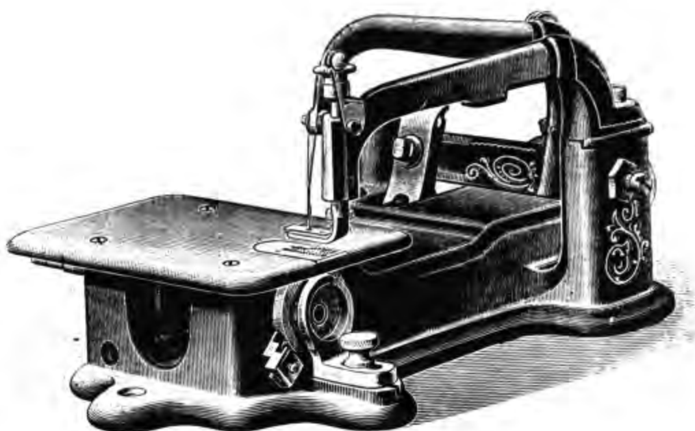
Figure 207.—SINGER SEWING MACHINE, 1924, manufacturing-machine class 1W, curved needle, is basically the Wheeler & Wilson sewing machine as manufactured by the Singer Company in the 1920s. It was designated "for fine lock stitching in the manufacture of shirts, collars, cuffs, etc." The machine head looks very much as it did in the 1860s. (Smithsonian photo 74-2123.)
