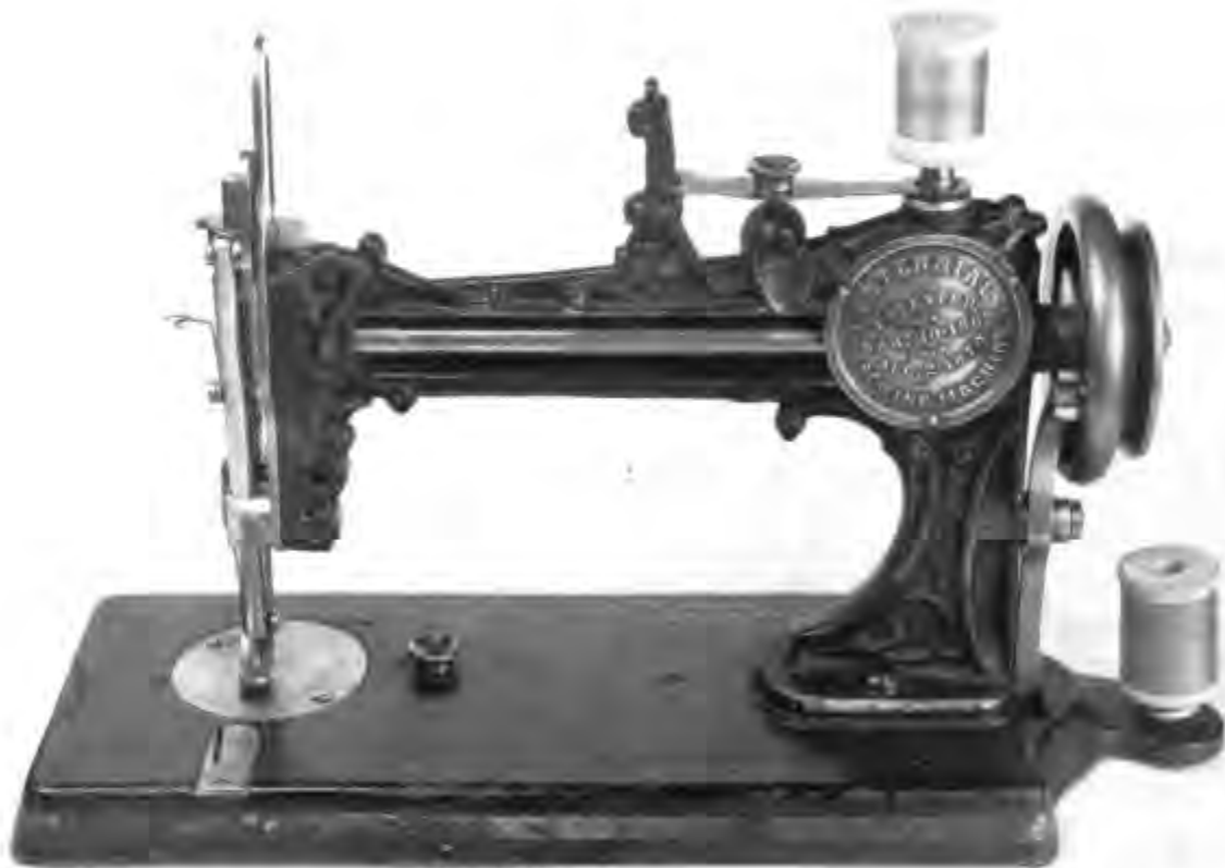
Figure 78.—CENTENNIAL SEWING MACHINE, 1876. The Centennial machine was basically a McLean and Hooper sewing machine which was renamed to take advantage of the coming Centennial celebration. It was based on the patents of J. N. McLean, March 30, 1869, and August 2, 1870, and made a two-thread chainstitch. Only about five hundred Centennial machines were manufactured in 1873, but by 1876 over three thousand had been constructed. The machines were advertised on white circulars which were printed in red and blue, and engraved with two women sewing, one by hand, labeled "Sewing in 1776," and one at a Centennial sewing machine, labeled "Sewing in 1876." There is no record that the machines were made after 1876. (Smithsonian photo 48216-T.)
