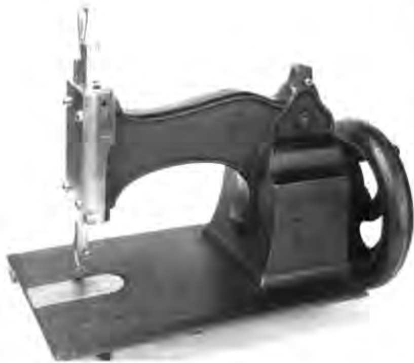
Figure 79.—CLARK'S Revolving-Looper double-thread sewing machine, 1860. This machine was manufactured by Lamson, Goodnow, & Yale of Windsor, Vermont. It was an attempt to improve on the combined ideas of the Grover and Baker machine, the Nettleton & Raymond machine, and the earlier single-thread Windsor machine. The improvements were made and patented by Edwin Clark on December 6, 1859. Widely advertised, the machines sold for $35 with a foot-power table. They could also be operated by hand. Over three thousand were manufactured and sold, and preparations were being made to continue manufacture of the earlier single-thread Windsor, originally made by the company's predecessor, Vermont Arms Co., when the Civil War broke out. A flood of arms orders arrived, and the sewing-machine manufacture was discontinued early in the summer of 1861. The sewing-machine equipment and business was sold to Grout & White of Massachusetts. (Smithsonian photo 48216.)
