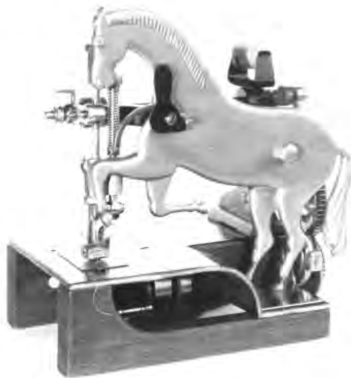
Figure 44.—THE HORSE SEWING MACHINE is among the most unusual of the patents issued for mechanical improvements. Although James Perry, the patentee, made several claims for the looper, feeder, and tension, he made no mention of the unusual design of the machine, for which a patent was issued on November 23, 1858. Although it was probably one of a kind, the horse machine illustrates the extent to which the inventor's mind struggled for original design. (Smithsonian photo 45505-C.)
