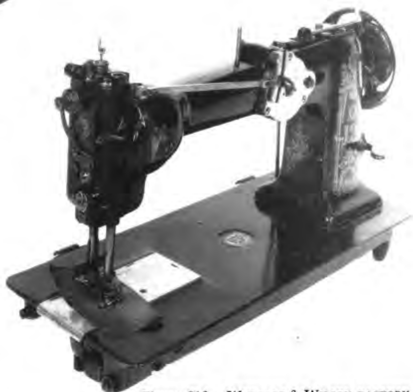
Figure 213.—WHEELER & WILSON FACTORY MACHINE of 1891 for a 3-stitch zigzag. (Smithsonian photo 73-11200.)
