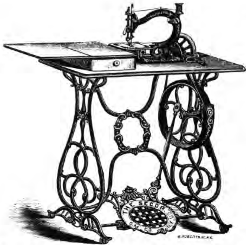
Figure 148.—THE SECOR LOCK-STITCH SHUTTLE SEWING MACHINE as illustrated in a broadside of about 1870. The name of the sewing-machine company cast into the treadle, or some other part of the framework, became increasingly common. (Smithsonian photo 67219.)
