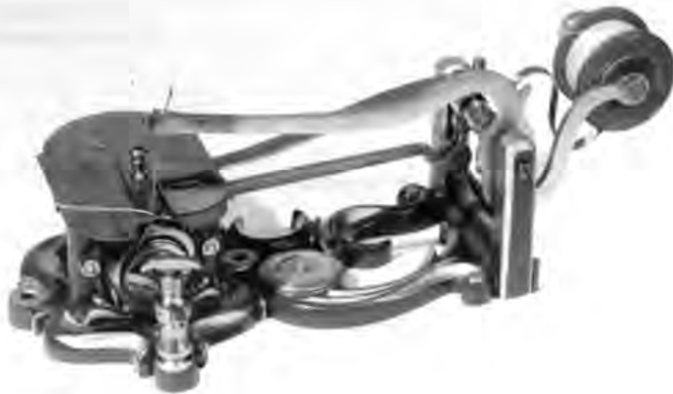
Figure 26.—WILSON'S stationary-bobbin patent model, 1852; a commercial machine was used since Wheeler, Wilson, Co. had begun manufacturing machines the previous year. (Smithsonian photo 45504-B.)
