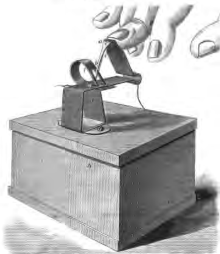
Figure 49.—HEYER'S MACHINE as illustrated in Scientific American , July 30, 1864. The smallest and most original of all the attempts to simplify machine sewing, Heyer's machine, which made a chain-stitch, was constructed of a single strip of metal. The Scientific American stated: "It is simply a steel spring ingeniously bent and arranged and it is said to sew small articles very well. The whole affair can easily be carried in the coat pocket."
