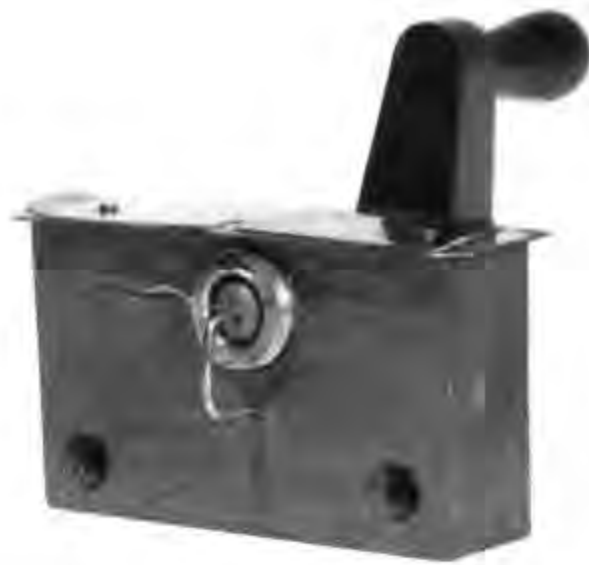
Figure 24.—WILSON'S PREPATENT MODEL for his rotary hook, 1851. (Smithsonian photo 45506-E.)
