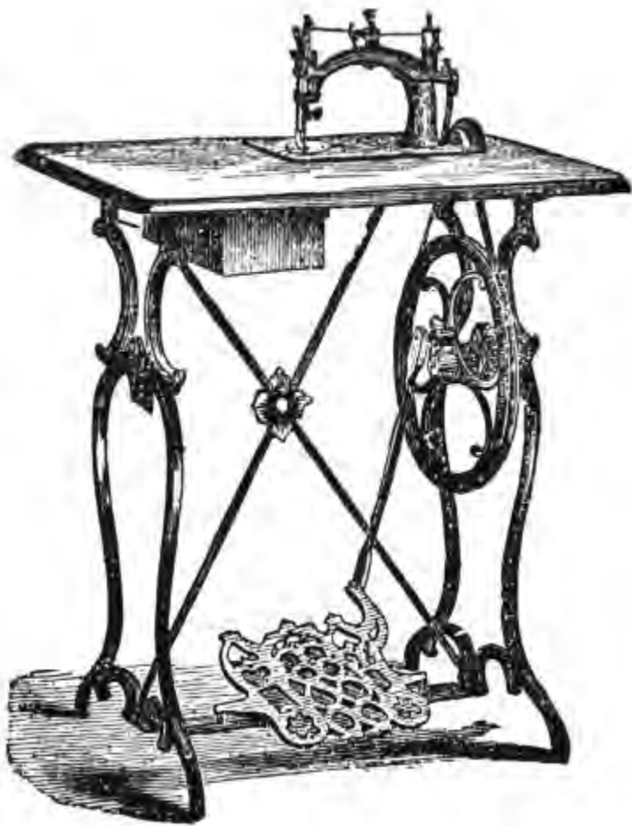
Figure 163.—THE INDEPENDENT NOISELESS FAMILY SEWING MACHINE sold for $50 about 1875. The legs are cast in a design similar to the early Wheeler and Wilson machines. (Smithsonian photo 67221.)
