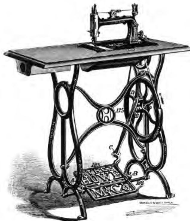
Figure 168.—THE NEW 'B' HOWE SEWING MACHINE as illustrated in an instruction book of about 1877. Minor changes in machine frame and the addition of a stitch-size regulator distinguishes it from the Howe machine of 1870 (see fig. 98). (Smithsonian photo 67206.)
