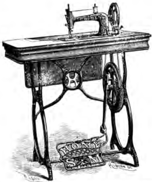
Figure 151.—THE HOME SEWING MACHINE of about 1870 shows one of the many head styles that is quite similar to the Singer family machines. (Smithsonian photo 67203.)
