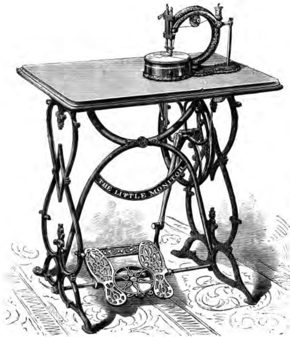
Figure 80.—DU LANEY SEWING MACHINE of about 1872. Most of the small, simple, chainstitch sewing machines of this period were constructed so that they could either be turned by hand or set into a treadle-powered table. Du Laney's Little Monitor, manufactured for only a few years, was based on the patents of G.L. Du Laney, July 3, 1866, and May 2, 1871. It was a two-thread, chainstitch machine powered only by a foot treadle. By simple adjustment, the machine could also make the cablestitch and the lockstitch. (Smithsonian photo 48221-C.)
