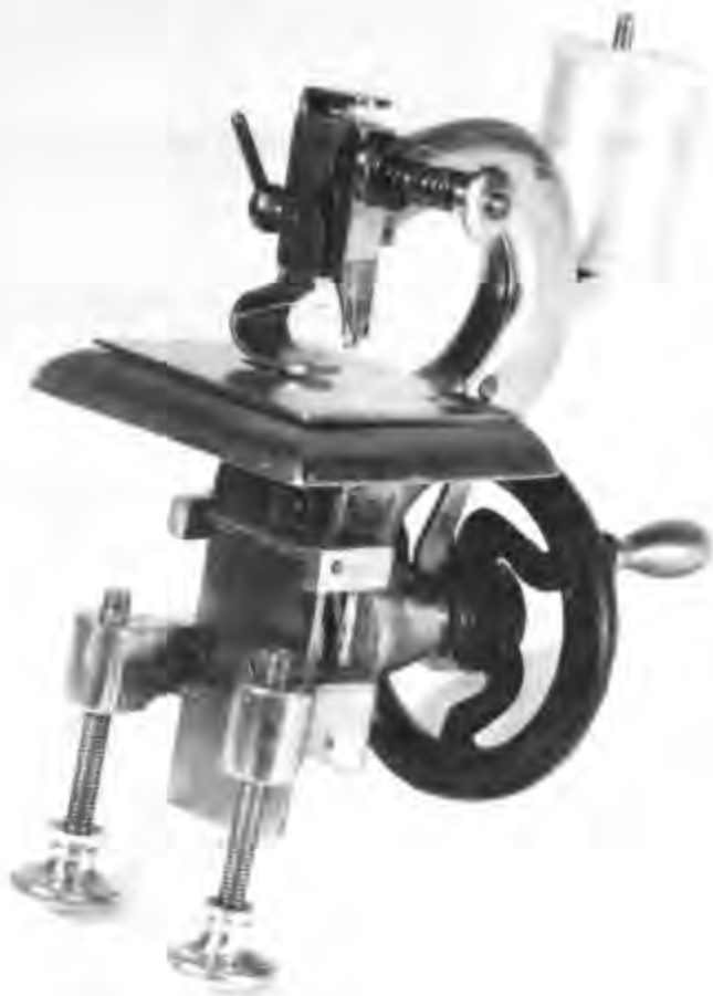
Figure 45.—MANY INVENTORS attempted to cut the cost of manufacturing a complicated machine. One of these was Albert H. Hook, whose machine is only about four inches high and two inches wide. His patent, granted November 30, 1858, simplified the construction and arrangement of the various parts. Although Hook used a barbed needle reminiscent of the one used by Thimonnier, his method of forming the stitch was entirely different. The thread was passed through the necessary guides, and when the cloth was in place the needle was thrust up from below. Passing through the fabric, the needle descended, carrying with it a loop of thread. As the process was repeated, a chainstitch was formed with the enchainéd loop on the under side. In spite of its simple mechanism, Hook's machine was not a commercial success. (Smithsonian photo 45505-D.)
