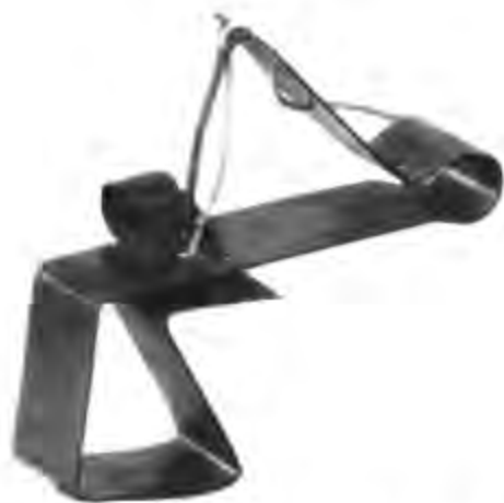
Figure 48.—HEYER'S POCKET SEWING MACHINE patent model, November 17, 1863. This patent model is one piece, and measures about two inches in height and two inches in length. It will stitch—but only coarse, loosely woven fabrics. As can be expected, a great deal of manual dexterity is required to compensate for the omission of mechanical parts. Heyer advertised patent rights for sale, but evidence of manufactured machines of this type has yet to be discovered. (Smithsonian photo 18115-D[a].)
