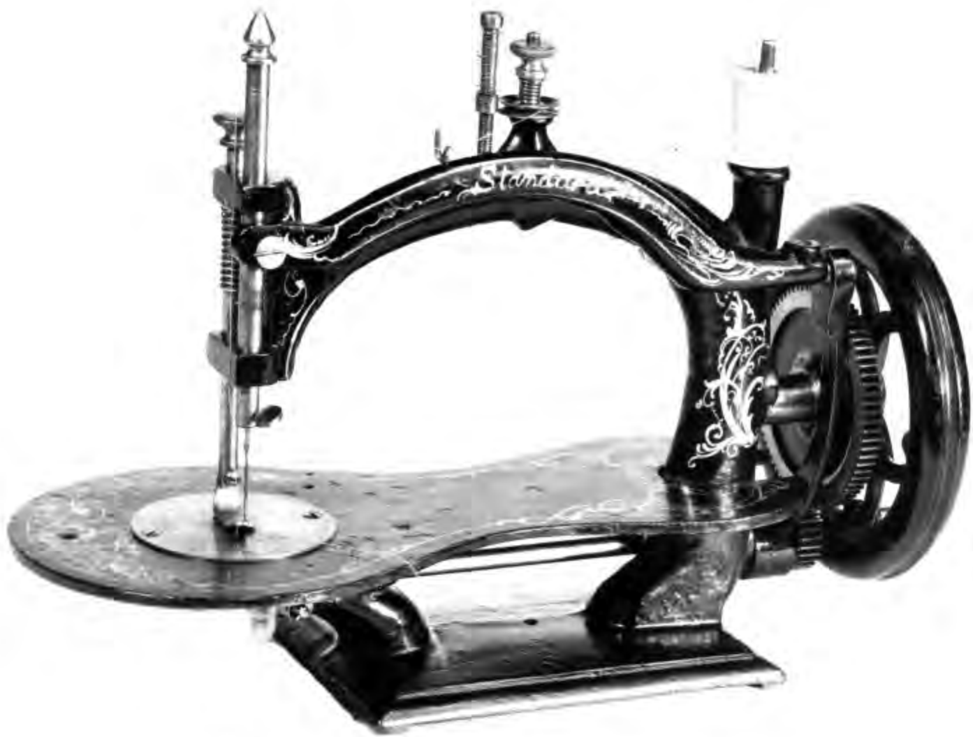
Figure 123.—STANDARD SEWING MACHINE of about 1870. This chainstitch machine is believed to have been made by the company that later became the Standard Shuttle Sewing Machine Company, when they began manufacturing lockstitch machines about 1874. This machine is marked with the name, "Standard," and with the dates "Patented July 14, 1870, Patented Jan. 22, 1856, Dec. 9, 1856, Dec. 12, 1865." The dates refer to the reissue and extended reissue of the Bachelder and the A. B. Wilson patents. The number of chainstitch machines of this type that were manufactured is not known. (Smithsonian photo 45506-C.)
