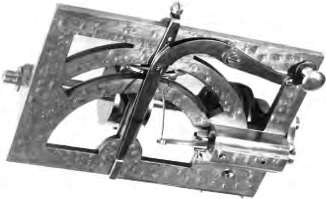
Figure 22.—WILSON'S PREPATENT MODEL for his reciprocating-shuttle machine, 1850. (Smithsonian photo 45525-A.)
