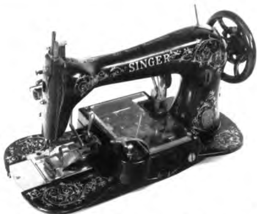
Figure 212.—SINGER FACTORY MACHINE of 1889 for making buttonholes has a device for cutting the buttonhole. Added in an 1890 patent is a mechanism for sewing on 4-eyed buttons for which Patent No. 425,422 was issued to J. P. Hallenbeck. (Smithsonian photo 73-11195.)
