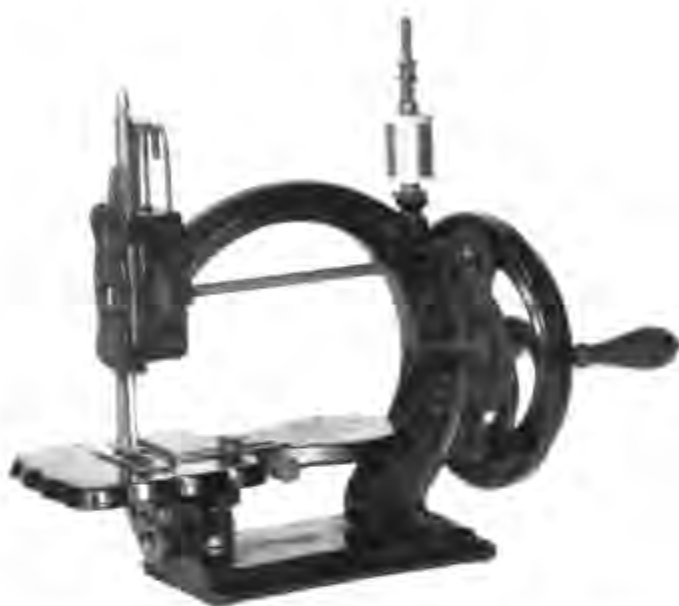
Figure 90.—GRANT BROTHERS SEWING MACHINE, 1867. This machine was one of several styles that utilized Raymond's 1861 patented chainstitch method. This machine, however, used an under feed rather than a top feed.
