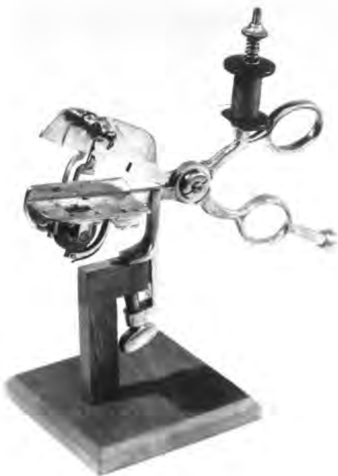
Figure 43.—THE SEWING SHEARS was another popular machine of unusual style. Some models were designed to both cut and sew, but most derived their names from the method of motivating power. The earliest example of the sewing-shears machine was invented by Joseph Hendrick, who stated in his patent that he was attempting to produce "a simple, portable, cheap, and efficient machine." His patent model of October 5, 1858, is illustrated. (Smithsonian photo 45504-F.)
