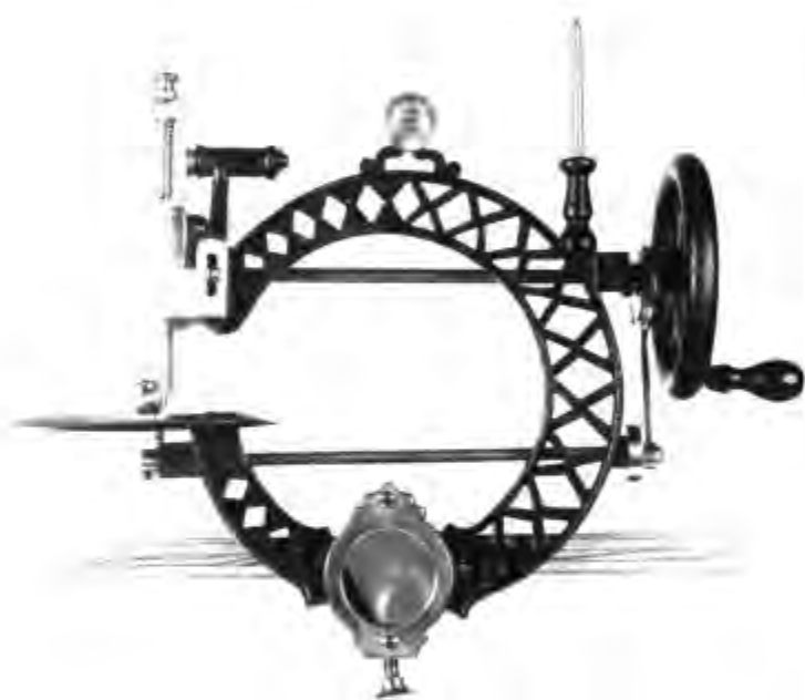
Figure 94.—HANCOCK SEWING MACHINE, 1868. Hancock in 1868 received both a design patent and a mechanical patent now using the eye-pointed needle and a hook to form the chainstitch. The design was an open framework circle with a mirror mounted in front of the table clamp. The purpose of the designated "looking glass" was decorative only. The Hancock machines were only manufactured for a few years. They measure 10\frac{1}{2} inches in width, slightly larger than the earlier machine. (Smithsonian photo 48328-M.)
