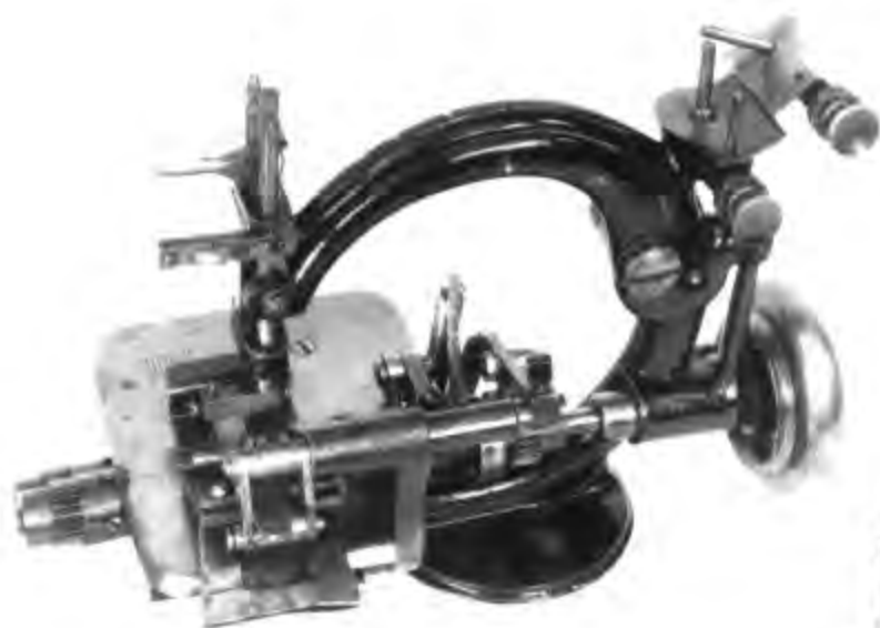
Figure 209.—WILLCOX & GIBBS FACTORY MACHINE for pleating and ruffling of 1874. Patent No. 156,119 was issued to Samuel Barney. (Smithsonian photo 73-11196.)
