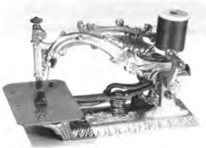
Figure 42.—THE FOLIAGE SEWING MACHINE originated with D. W. Clark. Once again he did not include the design in his June 8, 1858, patent, which was aimed at improving the feeding mechanism. Like most hand-turned models, these required a clamp to fasten them to the table when in operation. (Smithsonian photo 45504-C.)
