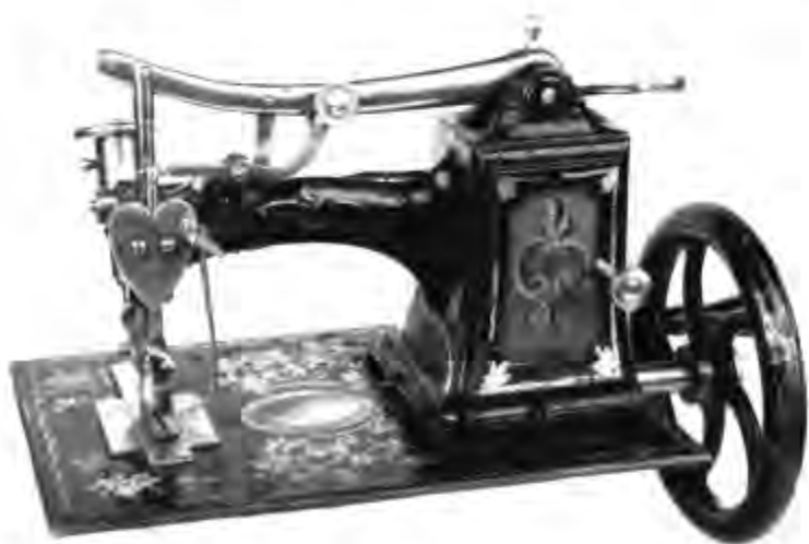
Figure 95.—[A.C.] HERRON'S PATENT SEWING MACHINE, 1858. The general style of this machine and the last Watson machines that sold for ten dollars are very similar. The Herron machines carried the patentee's improvement in the method of making the chainstitch and bore a small heart-shaped brass plate marked "A. C. Herron's Patent Aug. 4, 1857." The machines were provided with a hand crank, but were also meant to be operated by a belt and treadle. This machine head measures 14 inches wide. The manufacturer of this machine is not known, but it may have been produced by Watson & Wooster also. No records of the extent of manufacture of the Herron machines have been found. (Smithsonian photo 48329-J.)
