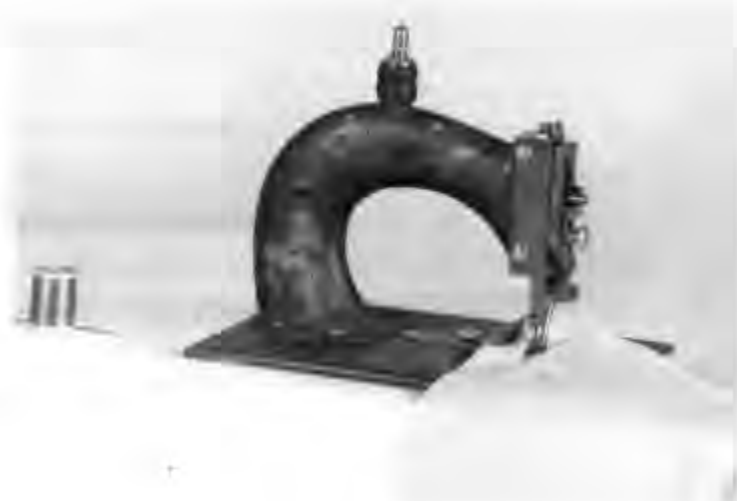
Figure 76.—BOUDOIR SEWING MACHINE, 1858. This machine, a single-thread, chainstitch model was based on the patents of Daniel Harris, dated June 9, 1857, June 16, 1857, and October 5, 1858. Manufactured primarily by Bennett in Chicago in
