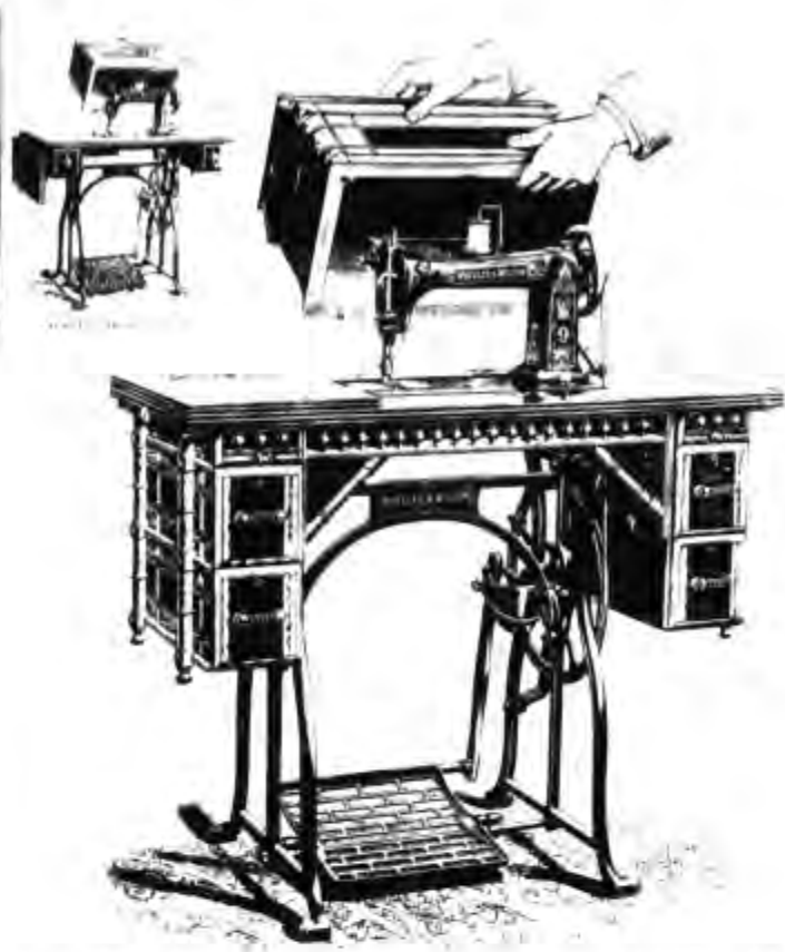
Figure 194.—WHEELER & WILSON SEWING MACHINE of 1891 showing a later style addition in the form of a spindle detail in the cabinet (see fig. 191). (Smithsonian photo 74-2100.)
