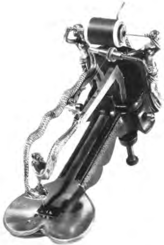
Figure 46.—IN ADDITION TO MECHANICAL PATENTS, a number of design patents were also issued for sewing machines. These fall into a separate series in the Patent Office's numerical records. This unusual example featured two semidraped female figures holding the spool of thread, a mermaid holding the needle, a serpent which served as the presser foot, and a heart-shaped baster plate. The design was patented by W. N. Brown, October 25, 1859, but no examples other than the patent model are known to have been made. (Smithsonian photo 45504-A.)
