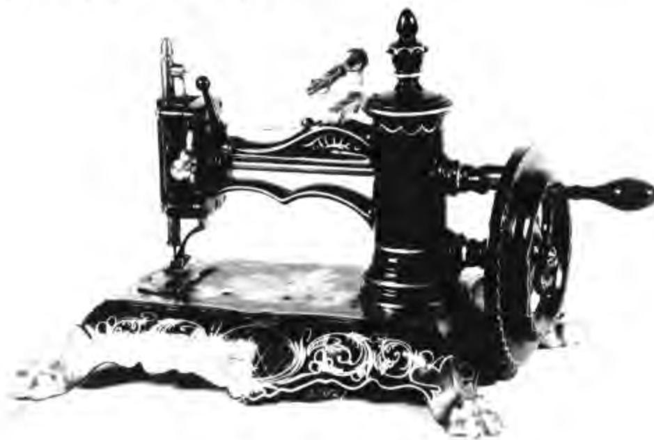
Figure 89.—WILSON SEWING MACHINE, late 1860s to early 1870s. In addition to the Buckeye (see fig. 77), W. G. Wilson manufactured several other styles of sewing machines. This one, a combination of the varying styles of the earlier pillar machine has even duplicated the general style of the spool holder patented by Folsom. The pillar is not striated, but the machine does repeat the claw feet of the Atwater and Monitor machines. Wilson machines are usually marked "Wilson Sewing Mach. Manuf'g Co. Cleveland, Ohio, Ketchum's Patent April 28, 1863." The latter name and/or patent date are found on many of the machines of this general construction. The patent is that issued to Stephen C. Ketchum for his method of converting rotary motion into reciprocal motion. (Photo courtesy of The Henry Ford Museum and Greenfield Village, Dearborn, Michigan.)
