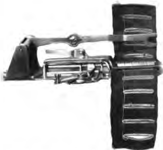
Figure 63.—HARRIS' patent buttonhole attachment, 1882. (Smithsonian photo P-63103.)
