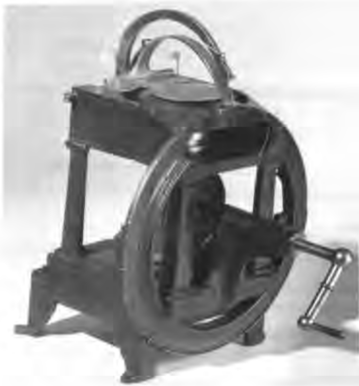
Figure 20.—BLODGETT & LEROW SEWING MACHINE, 1850, as manufactured by A. Bartholf, New York; the serial number of the machine is 19. The brass plate, serial number 119, at right, is from a later style of the same type of machine. (Smithsonian photo 48440-D; brass plate: 48440-K.)
