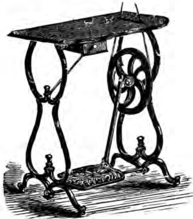
Figure 152.—A SEWING MACHINE TABLE of about 1870 sold to be used with the Buckeye sewing machine (fig. 77). Hand-turned sewing machines were frequently sold with or without tables, to be used as a hand machine or a treadle machine. (Smithsonian photo 67214.)
