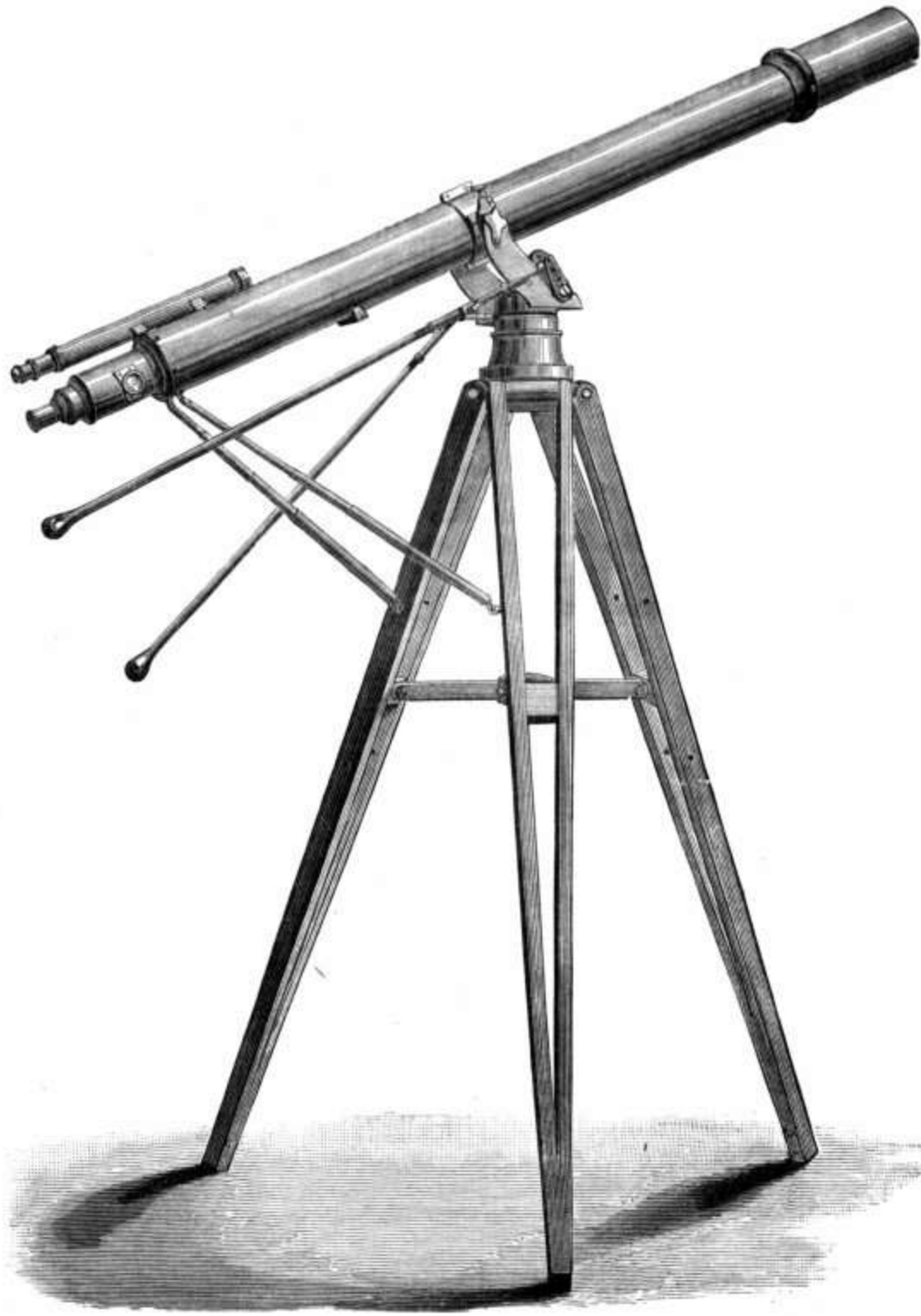
Portable Astronomical Telescope, with Alt-Azimuth Mounting.
