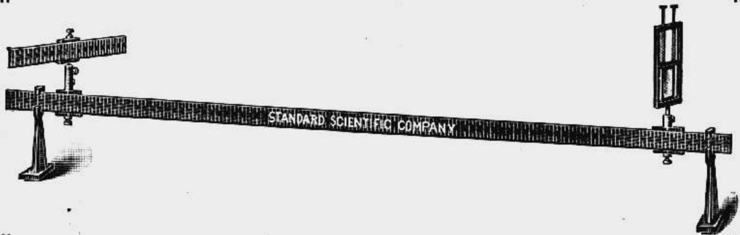
FIG. 4. WAVE-LENGTH OF LIGHT BY DIFFRACTION GRATING.
